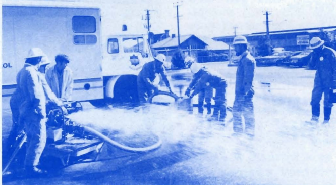
Learning about pumps—Students at the school involved in one of the practical sessions, operation of a GAAM 200 pump. Experimenting with flows and outputs.
